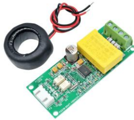
Gambar 1. Sensor PZEM-004T
